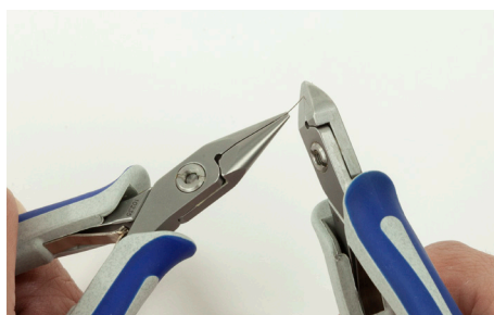
Cut a tip from Pt/Ir wire
