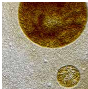
Lamellar structure of LDPE domains embedded in a polystyrene matrix. Image size 1 \times 1 \mu\text{m}^2
