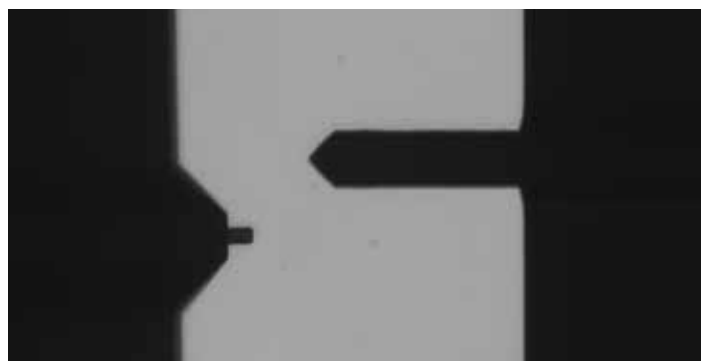
Comparison of a small and a conventional AFM cantilever. The small and regular cantilevers have tip view dimensions of 10\ \mu\text{m} \times 20\ \mu\text{m} (w x l) and 27\ \mu\text{m} \times 150\ \mu\text{m} (w x l), respectively.
