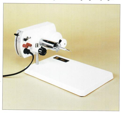
Doses from 0.1 to 10 ul. in twenty steps can be rapidly selected. The instrument may be used in any position, while low voltage and power consumption enables it to be operated from mains or battery using a foot or ring and finger switch.
