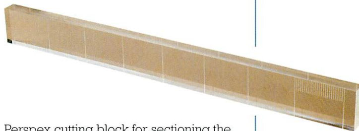
Perspex cutting block for sectioning the Melinex tape into hourly/daily samples
