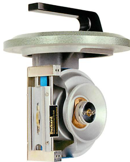
Alternative lid assembly for 24 hour sampling directly onto glass slide
