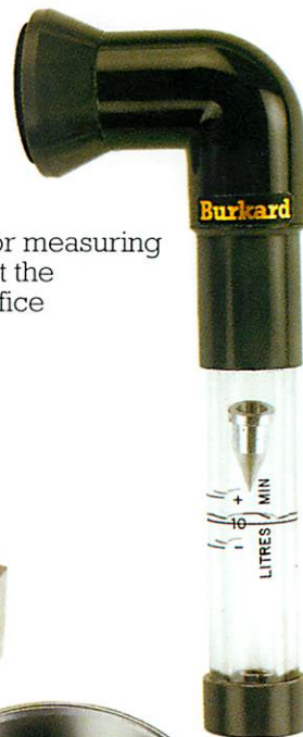
Alternative lid assembly for 24 hour sampling directly onto glass slide
