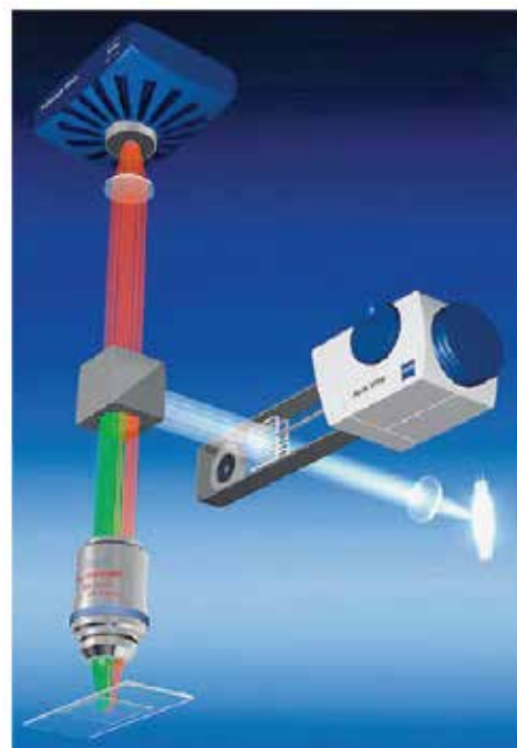
Figure 5: Structured illumination with the ApoTome. The slider contains a glass plate with a vapor-deposited grid structure and a plane-parallel glass plate which can be tilted by means of a galvo scanner mechanism.
