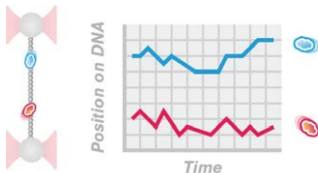
Figure 1b: A schematic illustration describing Cas9's binding by time-binning the intensity of the cyanine-derived fluorescence on the DNA molecule using data from a kymograph.
