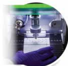
TLC/CMS – mass analysis of TLC spots
